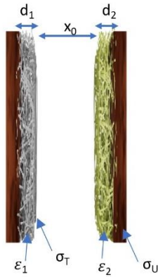
Figure 21: Representation of parameters for theoretical calculation with DDEF model.
