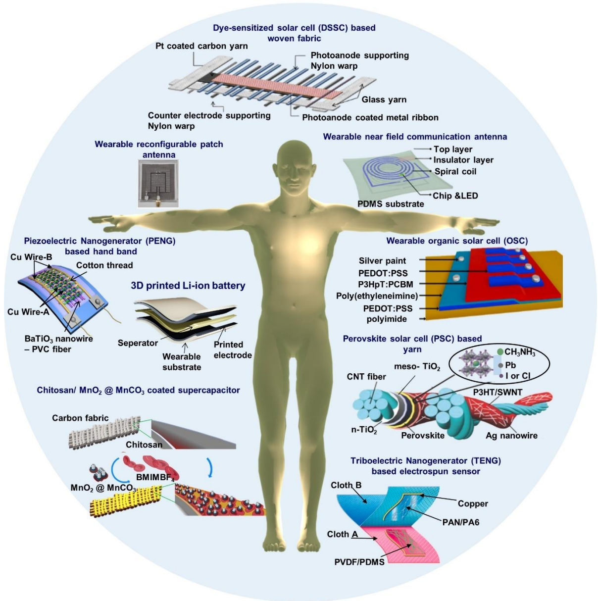
Figure 1: Examples of recent developments in energy autonomous wireless sensing devices including wearable energy harvesting, self-powered sensing, energy storage and communication devices.
