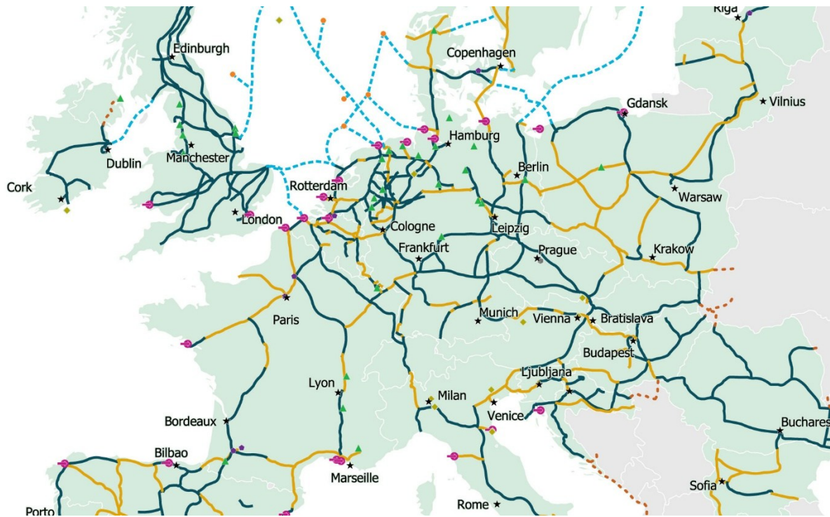
Figure 22 European Hydrogen Backbone pipe network
