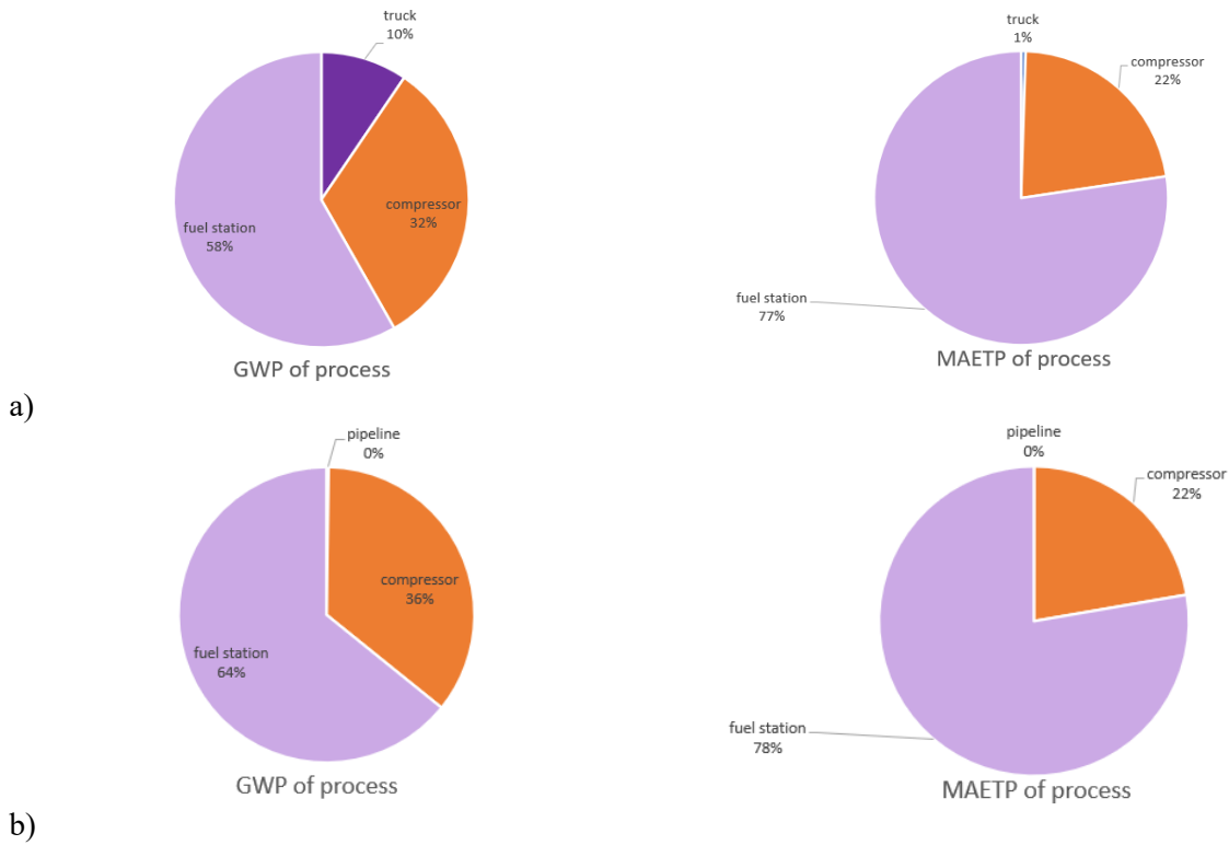
b) Figure 34 Comparison of GWP and MAETP contributions across hydrogen delivery processes by a) truck and, b) pipeline
