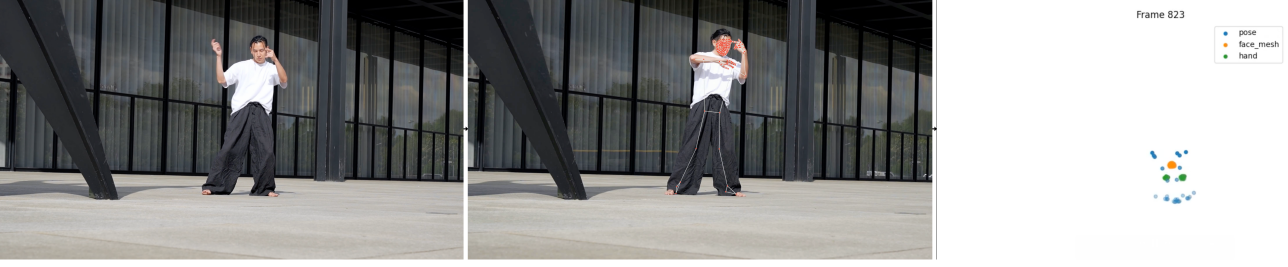
Fig. 3. Visual representation of the holographic preprocessing pipeline. The first image shows the original video frame, the second image overlays the landmarks extracted using MediaPipe Holistic (face, hand, and pose), and the final image displays the 3D point cloud segmentation of the same frame showing individual segments (face mesh in orange, hands in green, and pose in blue). This pipeline forms the foundation for further 3D reconstruction and streaming.
