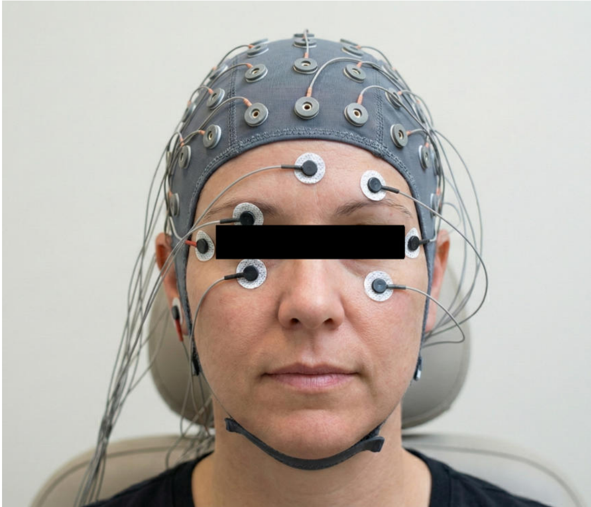
Figure 2.2: Example EEG and ocular electrode montage. The participant wears a 32-channel EEG cap together with horizontal and vertical EOG electrodes, periocular EMG electrodes and their associated ground/reference electrodes around the eyes and face. This configuration provides high-quality ocular signals but increases setup time and can be uncomfortable or visually intrusive for users, especially outside controlled laboratory settings.
