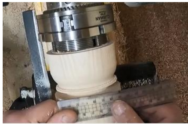
Figure Six: Measuring The Size Of The Tenon
