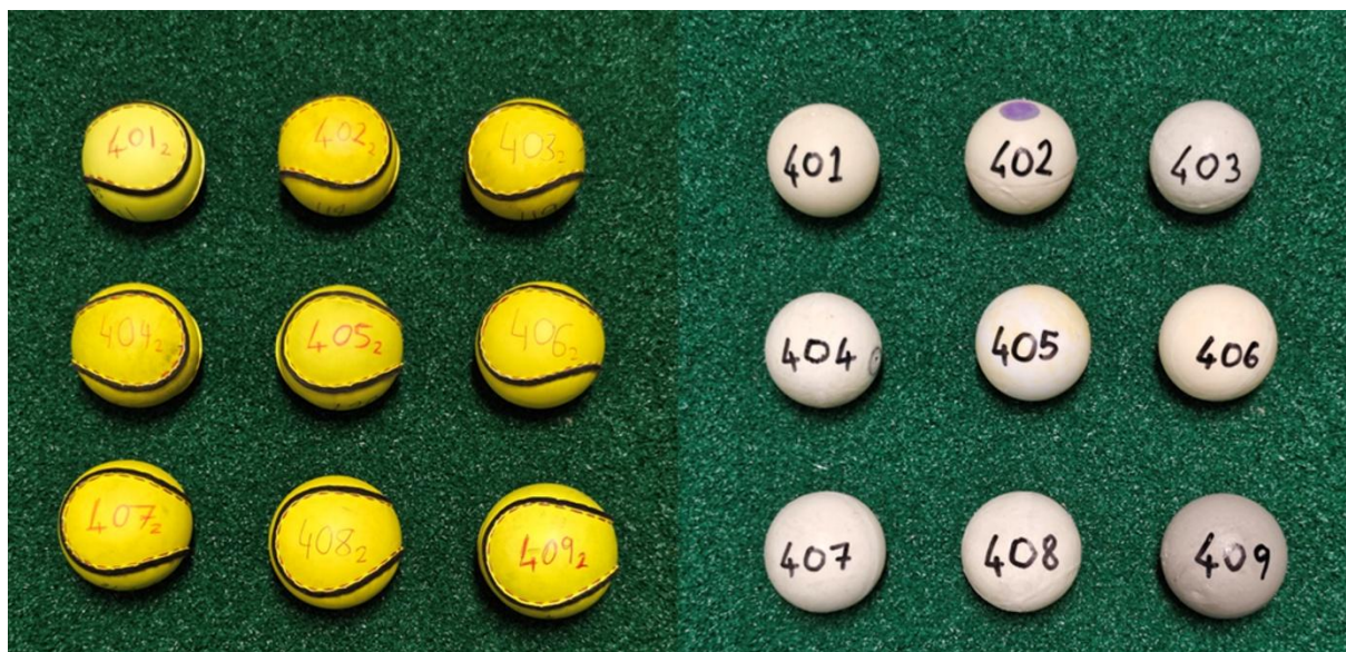
Fig. 2: Picture showing the test sliotars with marked sample numbers 401-409 and the same sliotars showing the core with leather covering removed.
