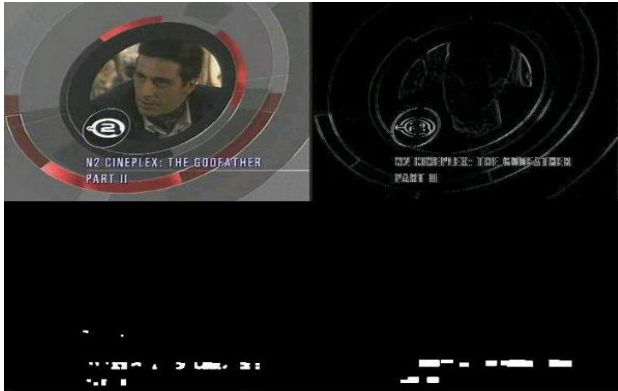
Fig. 2. (a) Input image, (b) horizontal difference magnitude, (c) (d)binarised edge map before and after morphological processing frame. As can be seen from Figure 2, the binarised edge map contains some noise pixels. In order to remove these, several steps are taken. The first step is to use a 3x3 median filter that deals well with the noise spikes whilst preserving the edges. In the sample frame the benefit of median filtering in removing noise is not obvious as the noise spot is not a single pixel. However, its averaging effect is clear as the tiny black spots were removed from the white regions. The next step is a 3x1 dilation followed by a 5x5 opening. As can be seen in Figure 2, a 5x5 erosion succeeds in removing the noisy spot while the subsequent dilation with the same size structuring element restores the desired white clusters to their initial size.
