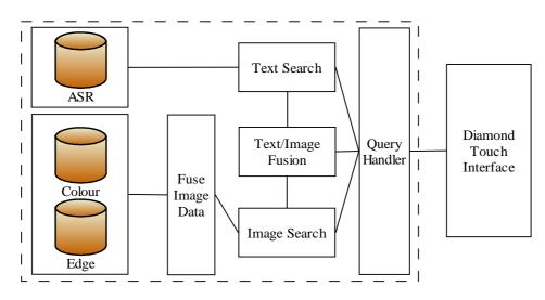
Figure 1: Físchlár-DT architecture
