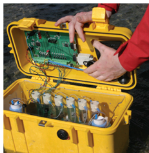
Figure 1: The phosphate analyser developed by CLARITY (left) and results over an 8-day period from a field trial at a waste water treatment plant (right) showing excellent agreement with a reference analytical system (total duration 49 days).
