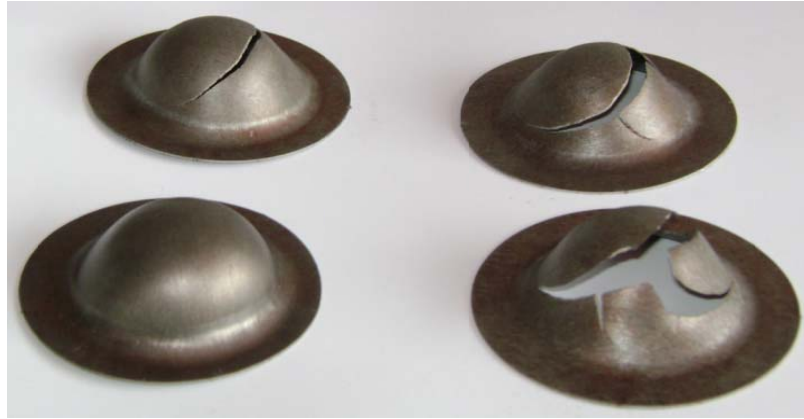
Figure 7-1: Bulged samples of Magnesium AZ31 formed at 100°C
