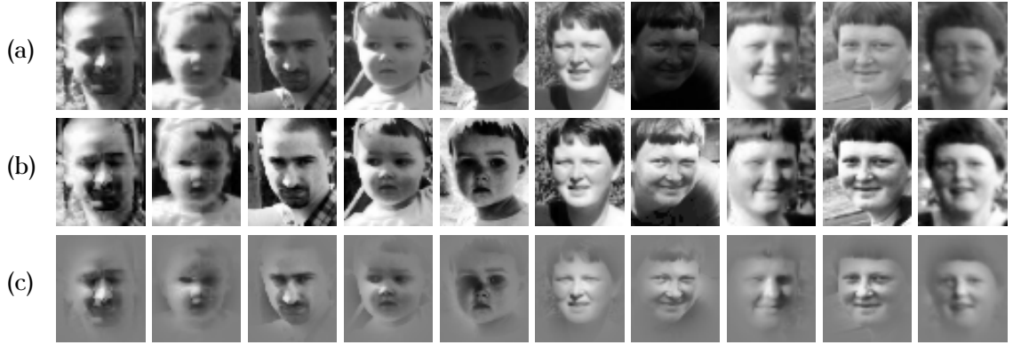
Figure 4.3: Examples of normalised facial image; (a) before any pre-processing, (b) after colour histogram equalisation, (c) after colour histogram equalisation and feathering with \sigma = 0.2 .
